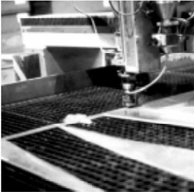
Fig 1. Aluminum cutting using CNC water-jet technology.
