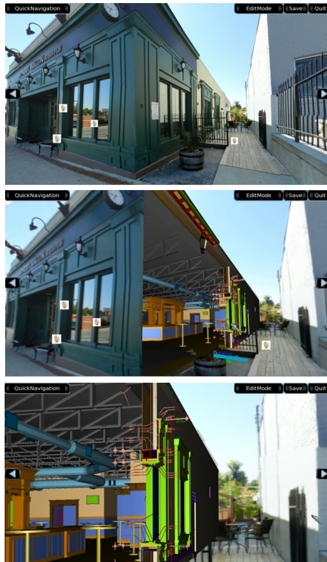
Fig. 4: Top: non-augmented scene. Middle: scene augmented with a clipped 3D model, revealing the inside of the building, which is further augmented with a 2D drawing. Bottom: detailed view.
