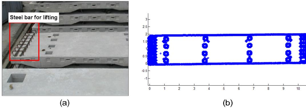
**Figure 5. Effect of external attachments on edge extractions: (a) A photo of steel bar for lifting; (b) The edge extraction result containing scan points of the steel bars**
