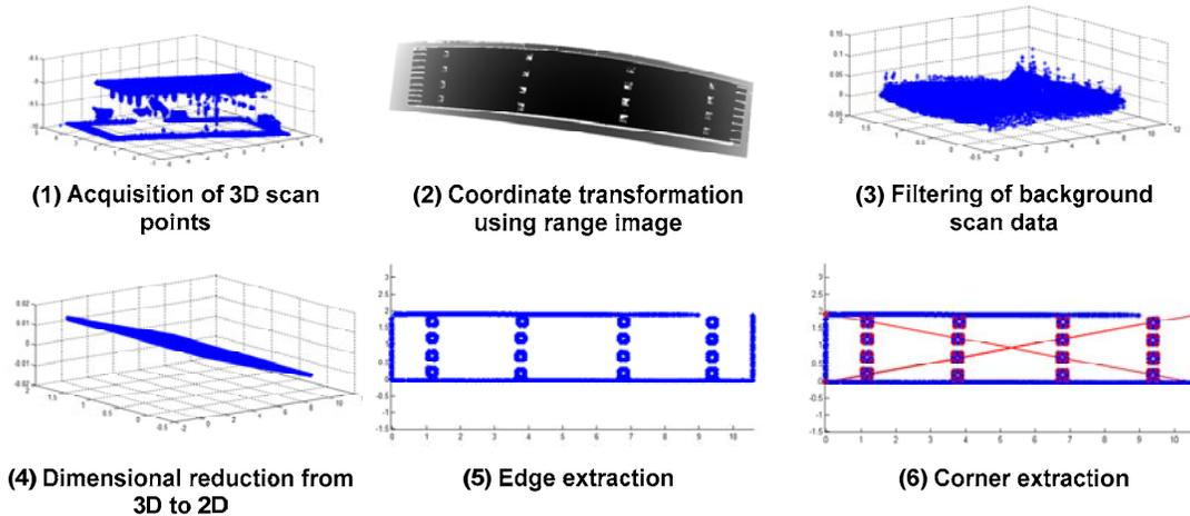
Figure 3. Data processing results of the field test
