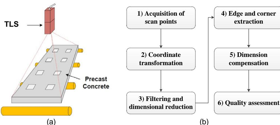
**Figure 1. Overview of the dimensional quality assessment technique for precast concrete panels: (a) Overall scheme; (b) Procedures of data analysis**
