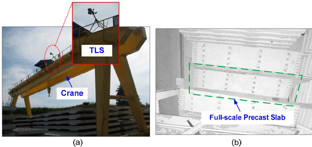
**Figure 2. Field test configuration: (a) Test set-up; (b) Top view of the inspected precast slab**
