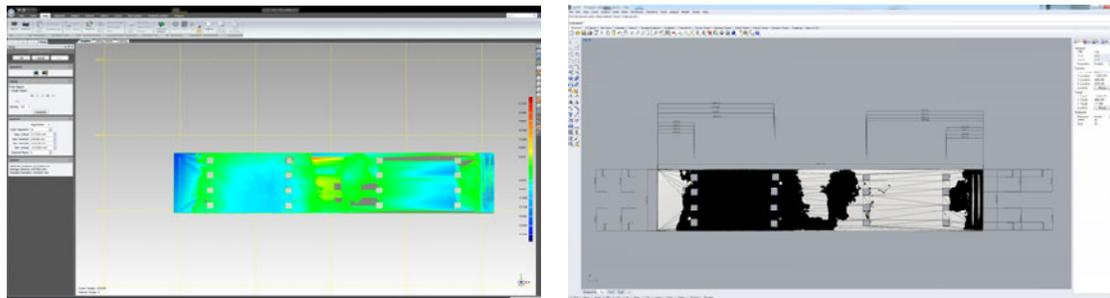
**Figure 6. Deviation analysis between design model and as-built model**
