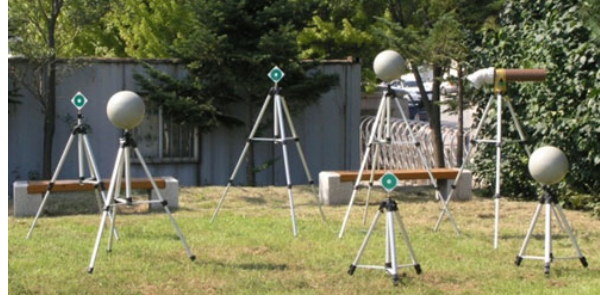
Figure 1. Array of Targets (planar, sphere, and pipe for accuracy check)
