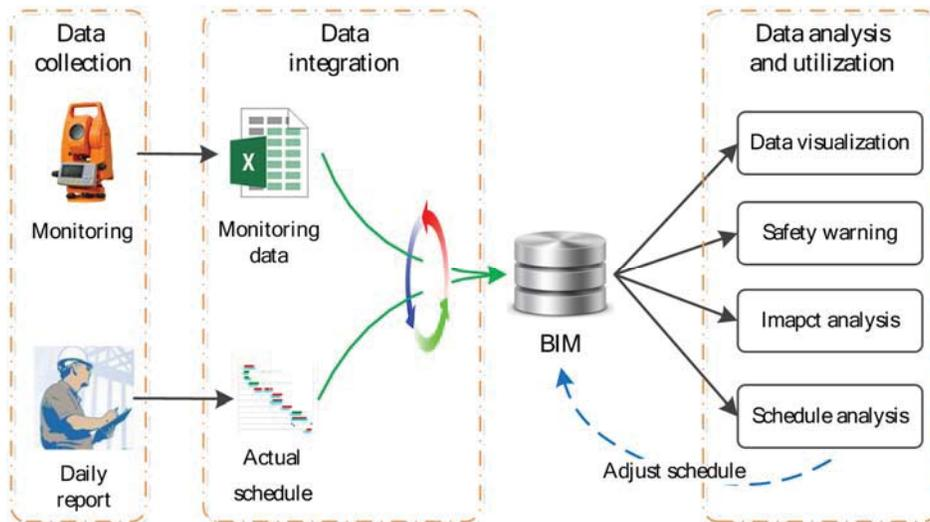
**Figure 3** Workflow for settlement monitoring and impact management
