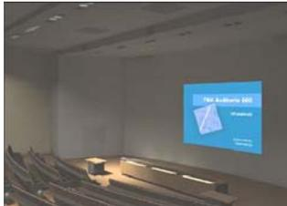
Abb. 5.46: LIGHTSCAPE renderings showed the end-user the proposed lighting designs for the auditorium hall in lecture mode (oben) and slide presentation mode (unten)
