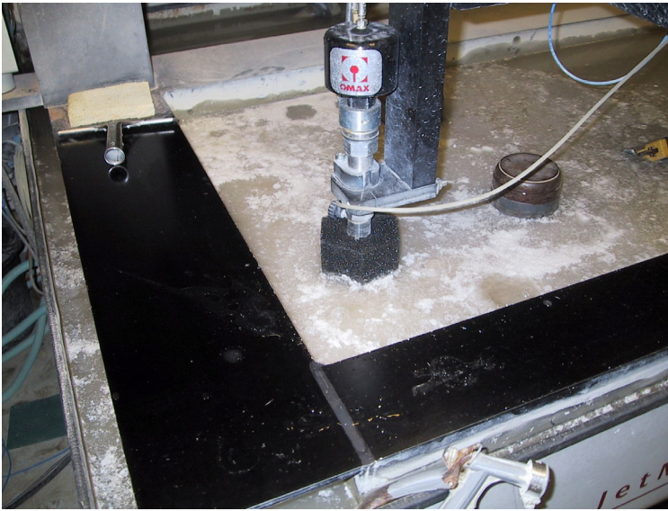
Figure 10. Cutting of the polycarbonate pieces in an OMAX™ water jet cutter
