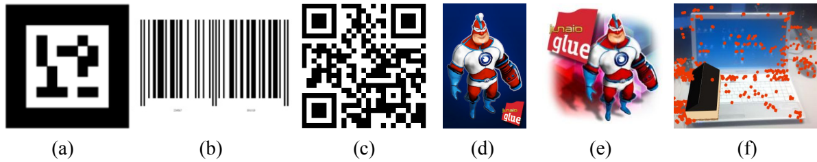
Fig. 3: Different types of AR markers for optical tracking (Metaio 2013): (a) ID marker, (b) barcode marker, (c) QR code marker, (d) picture marker, (e) markerless (borderless) marker, and (f) markerless 3D tracking.
