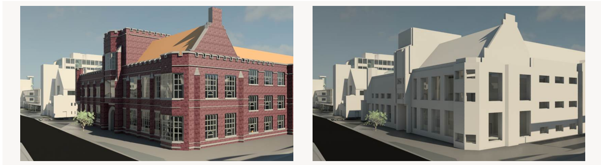
Fig. 7: a BIM model at AIA LOD 500 (left) and AIA LOD 100 (right)
