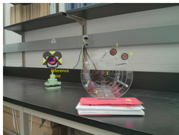
Fig. 6: The mockup TBM model for algorithm validation
