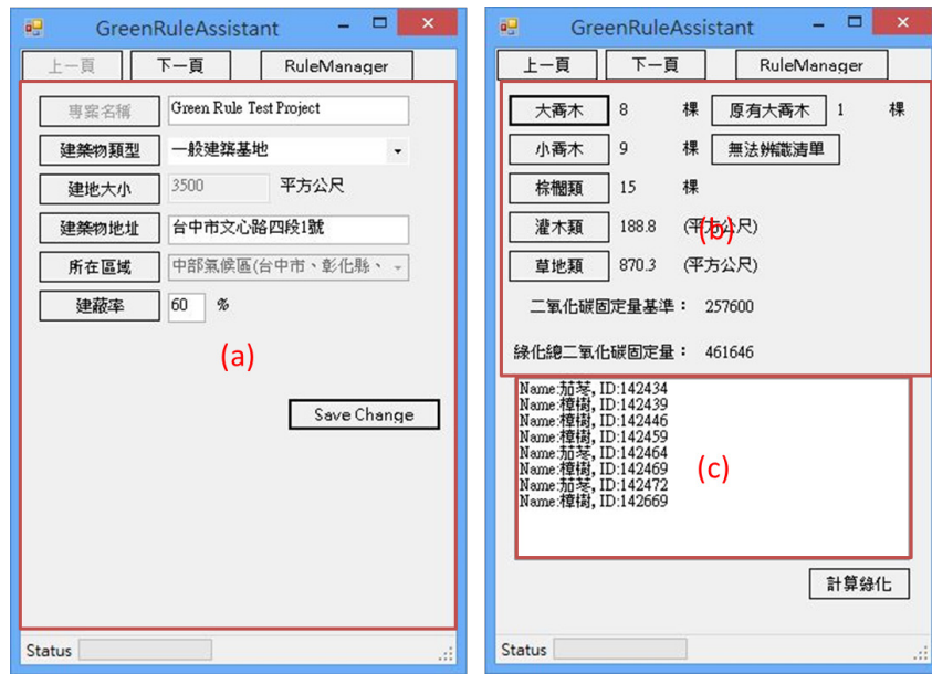
Fig. 3: GBDA's Revit User Interface: (a) building information, (b) evaluation result, and (c) object list display
