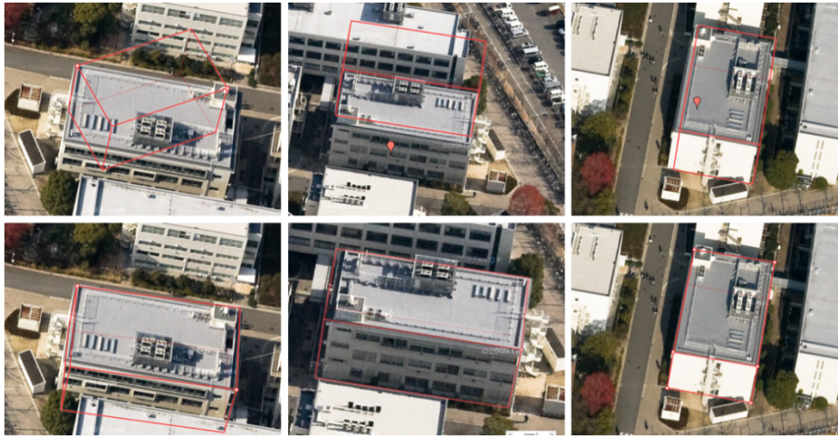
Fig. 1: Modeling process by Building Maker; Adjusting the size and positions of the bocks corners to that of building on the photos
