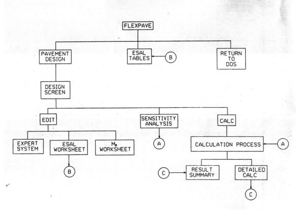
Figure 1 FLEXPAVE Flowchart
