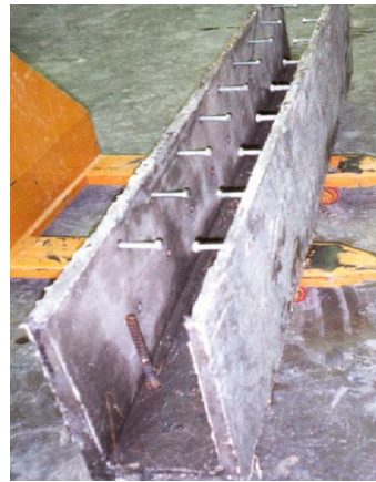
Figure 2. The 2.5 cm (1 in.) thick 1.52 m (5 ft) long, 40.6 cm (16 in.) high and 25.4 cm (10 in.) wide SIMCON stay-in-place formwork. Shear studs that were bolted directly into the formwork sides are clearly visible.
