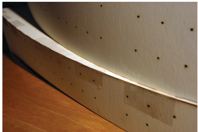
Figure 5: This prototype was exploring the accuracy of the finger joint method. This joint eased difficulty of fabricating the forms.
