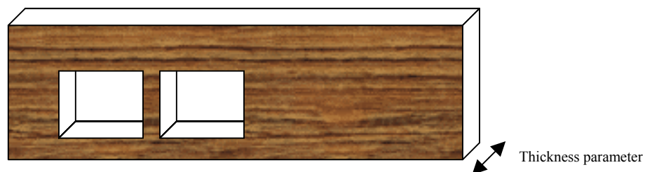
Figure 4. A 2.5D solid wall with window openings.
