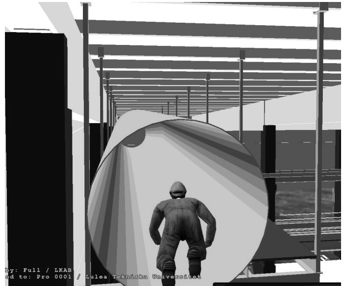
Figure 4. Screenshots extracted from a VR prototype describing how visual clash detections and spatial analyse of the installations with the help of an avatar was carried out.
