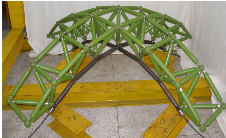
Photo 2: Deformed shape of Space Structure by means of Post-tensioning
