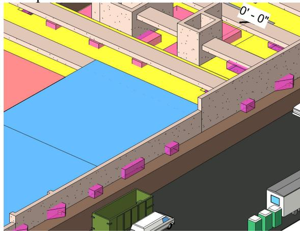
Figure 3: Object representing band beams, sub-grade, slab on grade and walls
