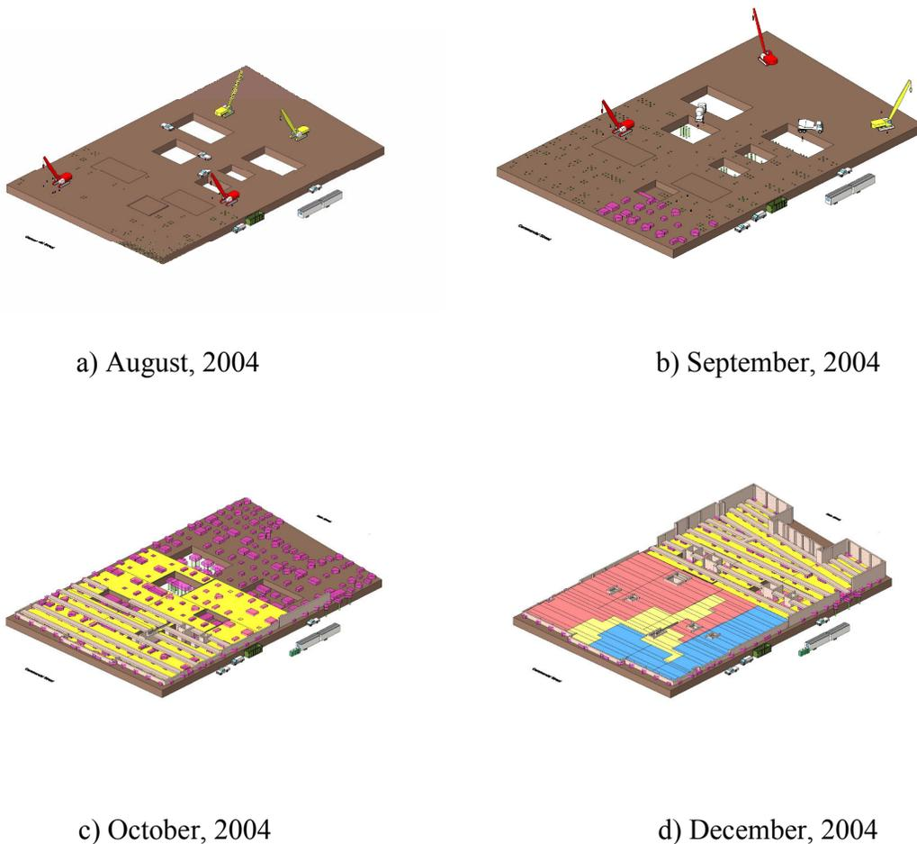
Figure 2: Gradual Progress of Site-Work and Foundations
