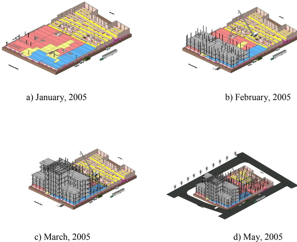
Figure 3: Gradual Progress of Steel Frame
