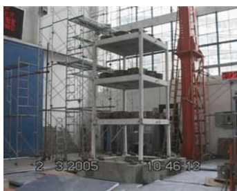
(a) Test model on the shaking table
