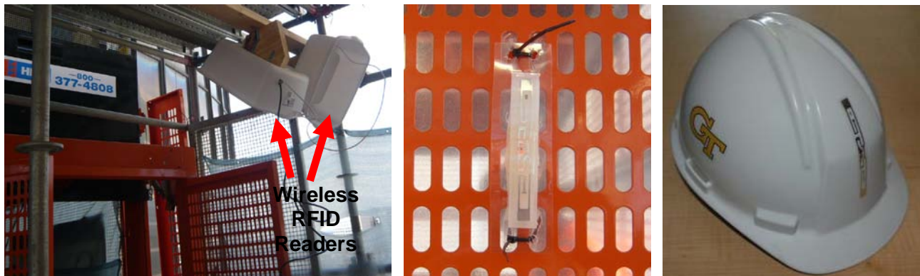
Figure 1: Wireless RFID reader on 16th floor, and passive RFID tags installed on buck hoist and worker helmet.
