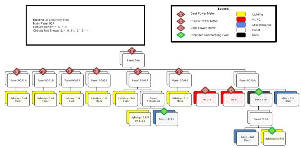
Figure 6 - Part of the electricity tree for Building 90, showing end uses and metered points
