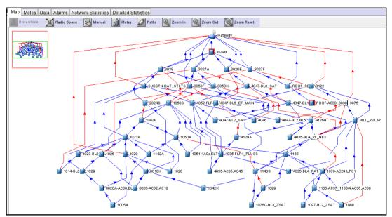
Figure 4 – Mesh instrumentation configuration for wireless sensing network
