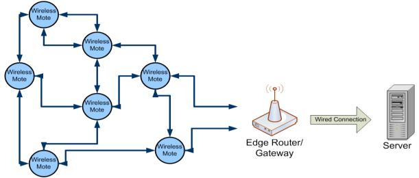
Figure 1: Wireless mesh network communication configuration
