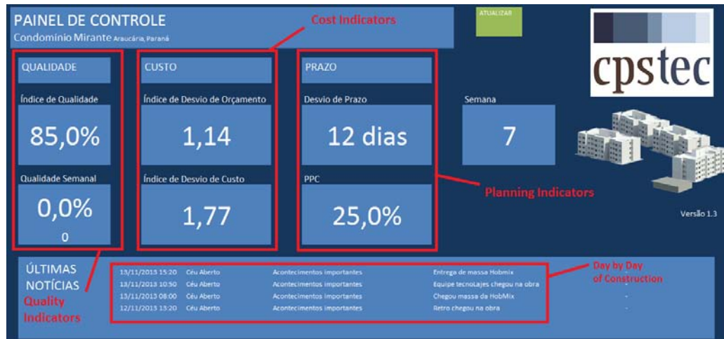
Figure 9. control panel: indicators to manage daily integrated with model.
