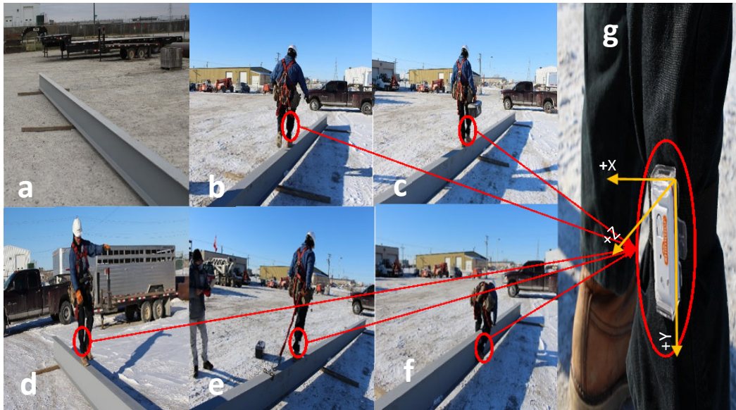
Figure 1. Illustration of the experiment: (a) I-beam used in the experiment; (b) walking at his comfort speed; (c) carrying a load on one side; (d) walking with a faster speed; (e) walking with a safety harness lanyard connected to the I-beam; (f) walking on the lower flange of the I-beam; (g) the IMU sensor attached to the right ankle of the ironworker.
