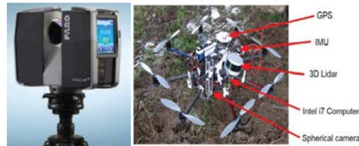
Figure 1: Figure depicting scanners (a) TLS (b) UAV
