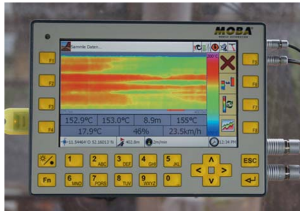
Fig. 71.2 Paver-mounted thermal imaging profile [6]
