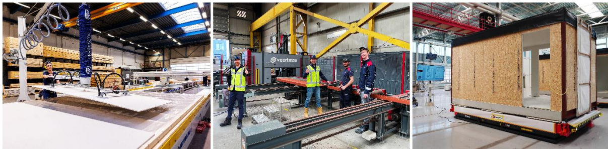
Figure 3. From left: timber framing robot, drilling machine, and a module on an Automated Guided Vehicle (AGV)
